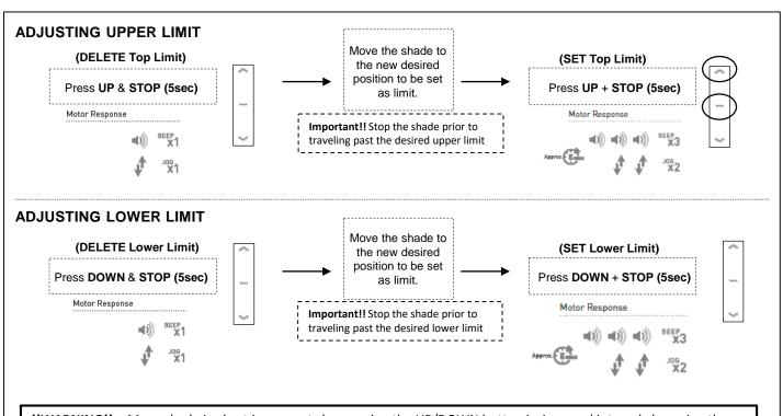
!!WARNING!! - Move shade in short increments by pressing the UP/DOWN button in 1 second intervals (pressing the UP/DOWN button for more than 3 seconds may send the shade past desired upper/lower limit and may result in damage to the product). Once you have reached the desired upper/lower limit, you can adjust the limit with either the UP and DOWN buttons. (remember to adjust in short increments!)
