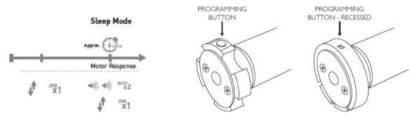
Note: Programming buttons will face down when shade is installed
