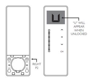
With the remote unlocked. Hold the UP and DOWN button on the controller for approximately 5 seconds. The motor will jog up and down once.
