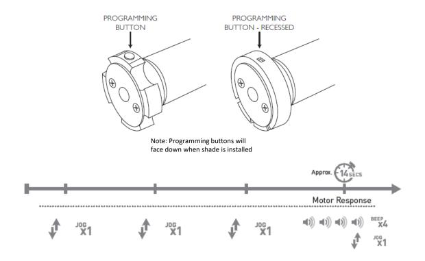
The motor will jog 4 times before the reset is complete. The P1 button must be held the entire time. 4 beeps confirm the factory reset is complete.
