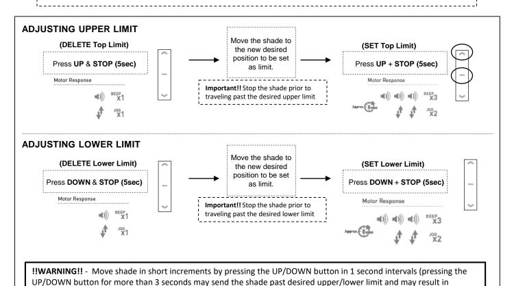
Once the limits have been adjusted as desired, return the remote control to "L" mode by pressing and holding the upper left P2 button under the battery cover. The other grouped motors can now be taken out of sleep mode by holding the programming button for 6 seconds
