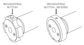
Note: Programming buttons will face down when shade is installed
