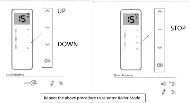
If you do not activate tilt mode in time the motor programming sequence will time out, repeat the above steps assuring to press the STOP button within 4 seconds of the motor jog
