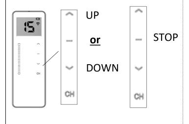
IF DIRECTION DOES NOT ALIGN WITH UP/DOWN BUTTONS – Press and hold down the UP <u>and</u> DOWN button simultaneously until the motor jogs UP and DOWN once.
