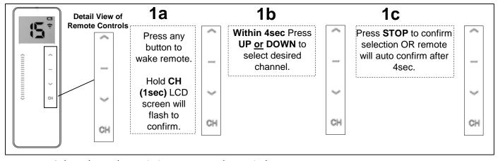
Note: Select channel on existing remote to be copied Select channel on new remote where existing channel will be copied
